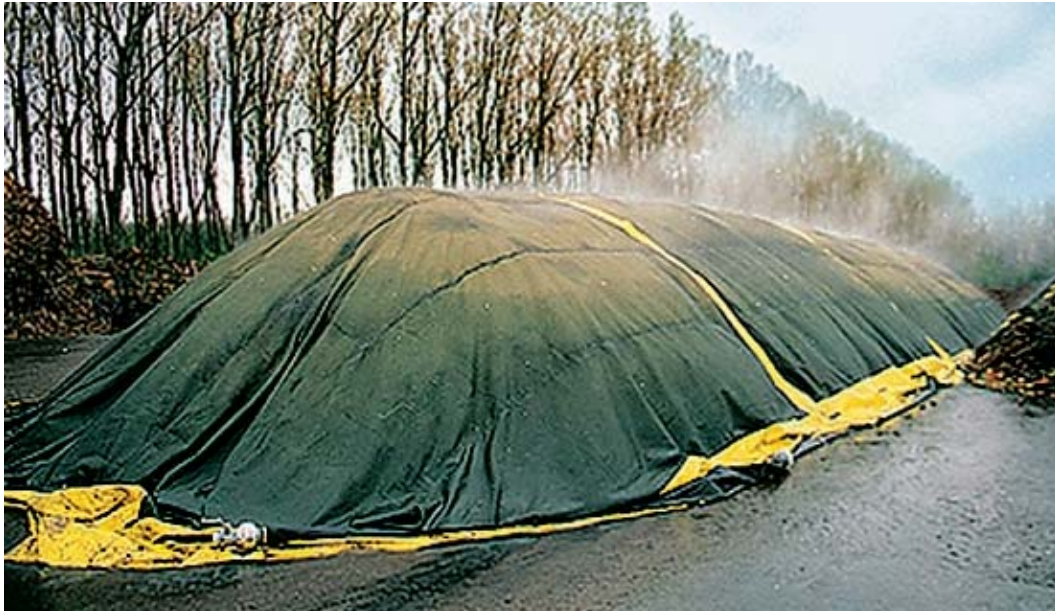
Figure 2: The GORE™ Covered Pile Static Composting System
